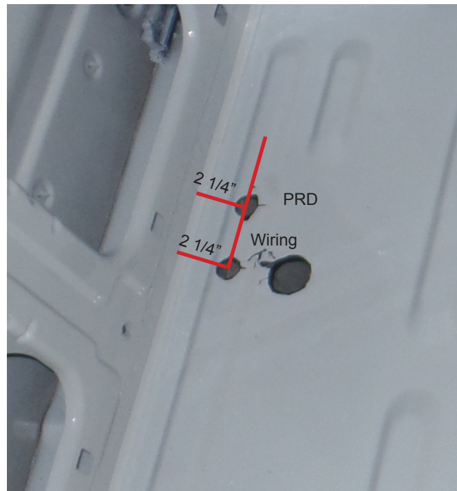
Center PRD and wiring holes on the first rib from the wall.
